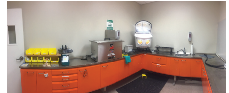
The WaterJet cleaning station removes support material without temperature cycling.
