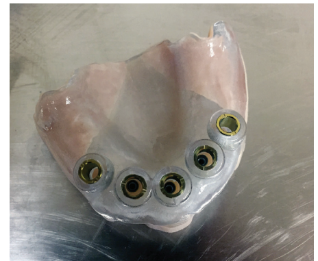
A drill guide printed in clear MED610 installed on dental model.
