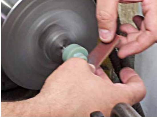
Figure 11: Finishing process of mold component.
